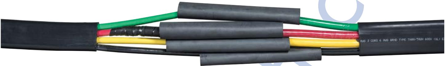
2nd Step: Wrap butt splices with self-vulcanizing rubber tape.
