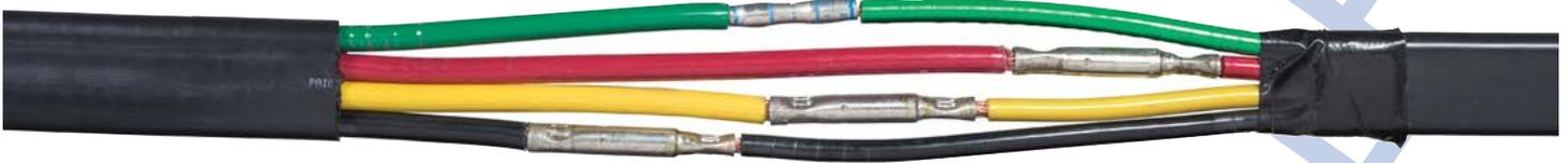
1st Step: Butt spliced together, crimp and solder
